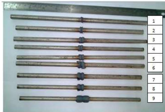
Figure 2: Friction Welded Samples.
